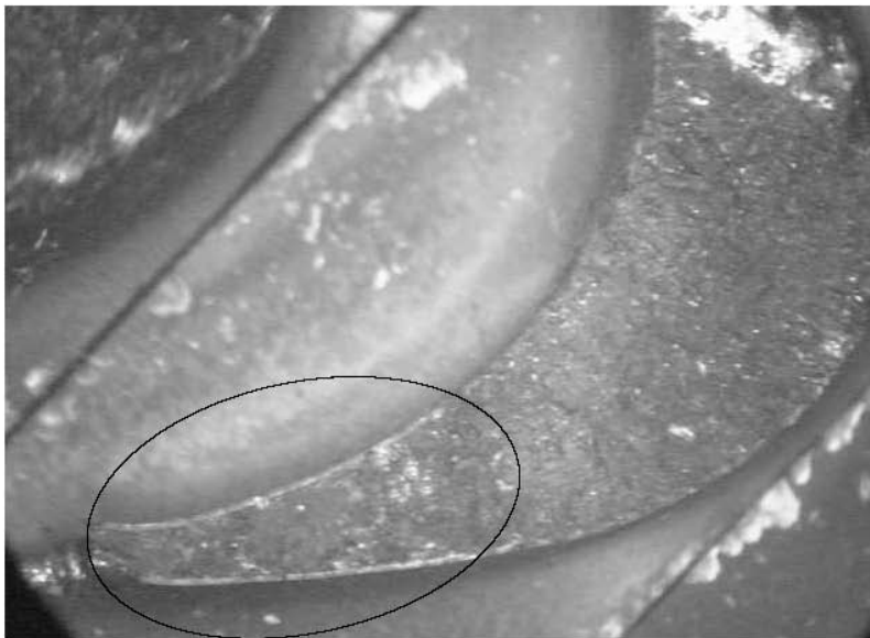
Photo No. 32 Magnified view of the circled region in Photo No. 31 showing a relatively flat fracture surface (circled). Impact damage has obliterated the T/E tip.
